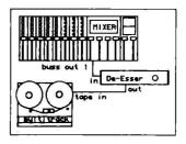
**Fig. 2:** Install a de-esser as the last processor in the chain before the recording device.
