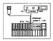
**Fig. 1:** Generally. a compressor limiter should patch into the insert of your microphone channel.
